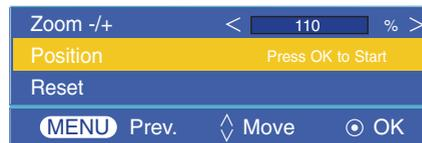
3. Press the  $\odot$  **OK** button. When the window below appears at the bottom right corner of the screen, press the  $\wedge$  /  $\vee$  /  $<$  /  $>$  to adjust the position. When the arrow turns black, maximum adjustment has been reached and no further adjustment can be made.
